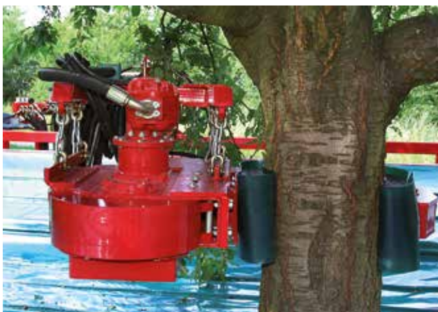
gripper – permits a gentle shaking – even after years there is no visible sign of where the gripper had enclosed the trunk
