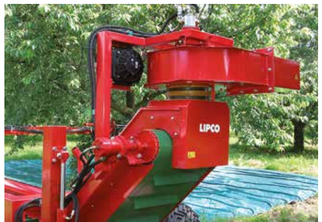
exhauster – separates even very dirty fruit completely from wood, leaves and other contaminants
