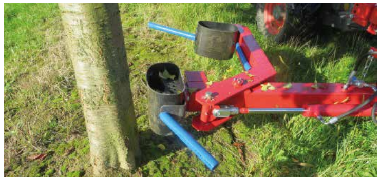
gripper can be folded
