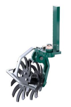
Integrated angle adjustment as is also the case with the disc harrow. The exterior angle can also be altered with no problems by reinserting the locking pins. Good distribution of force due to the different disc dimensions for the exterior and interior sprockets. As a result, both discs work in a sloped working angle at the same level. In comparison to the disc, we avoid creating a clear edge which can become a water channel on a steep slope.
