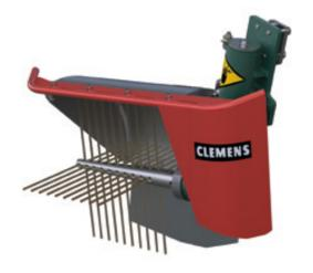
The mulching brush has very strong and smooth cords that protect the vine. The conical aluminum shaft operates smoothly and with little vibration because of its special shape. It is therefore possible to carry out weeding effectively at 1100 rpm. With the MULTICLEAN you can remove both the water shoots and the weeds simultaneaously with one machine.
