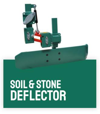
The soil & stone deflector is mounted behind the RADIUS to keep the cover crop clean of soil and stones. It comes with a parallelogram for ground adaptation. Different adjustment possibilities allow flexibility to achieve the desired results.
