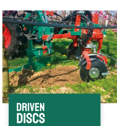
The discs (2 pcs.) are used to pull out soil of the vine interspace, for ploughing back or to ridge, for example for a better placement of slurry and dung. In addition to the sensor rod, the disc unit is equipped with a deflecting rail, which pushes the unit away from the vine in case the sensor rod is not triggered, thus preventing injuries and damages to the plant.
